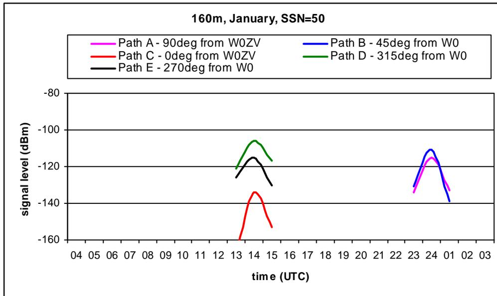
**Figure 1 – Signal Powers on 160m (using improved D-region model)**
