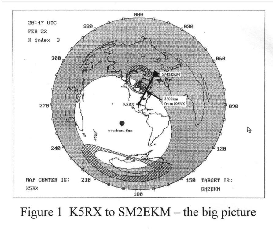
The first half of the path (the K5RX end) was in daylight. The last half of the path (the SM2EKM end) was in darkness, and went through the auroral oval tangentially.
