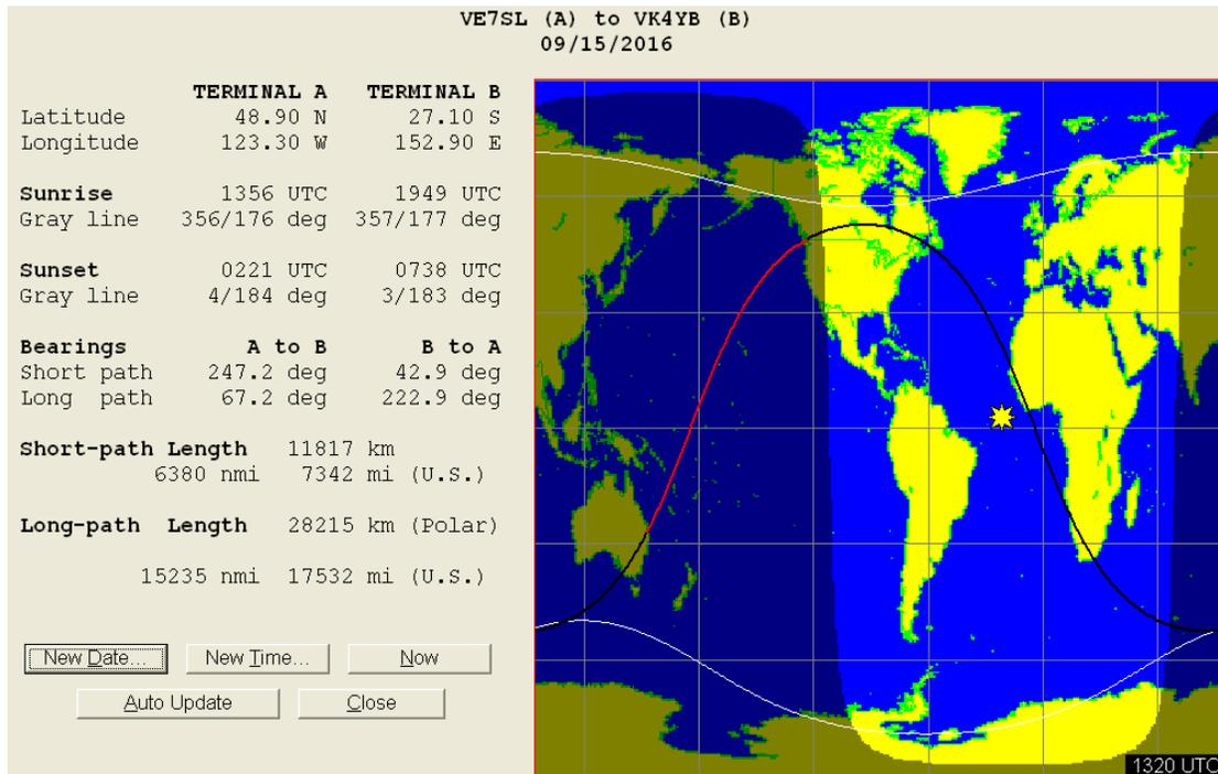
The red line is the short path between VE7SL and VK4YB. As expected, this QSO took place near sunrise on the eastern end of the path. On our low bands (especially 160-Meters), this condition can produce a sunrise enhancement in signal strength. It is likely to happen on 630-Meters, too.
