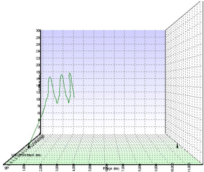
It looks like ducting in the nighttime electron density valley is a possibility for this QSO on 630-Meters. It should be noted that now the ordinary wave has excessive absorption, and the extraordinary wave is the likely candidate. I believe this is due to 630-Meters being below the electron gyro-frequency (the frequency at which electrons spiral around magnetic field lines).
