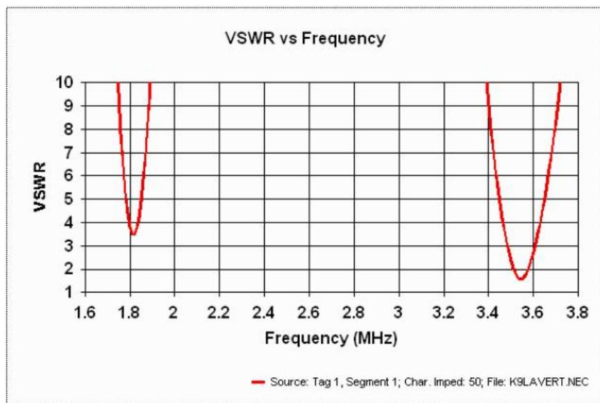
The impedance on 160m was around 15 ohms. After about 200 feet of RG-8 coax, the SWR was around 2.5:1 – my Commander HF-1250 amplifier had no problem loading
