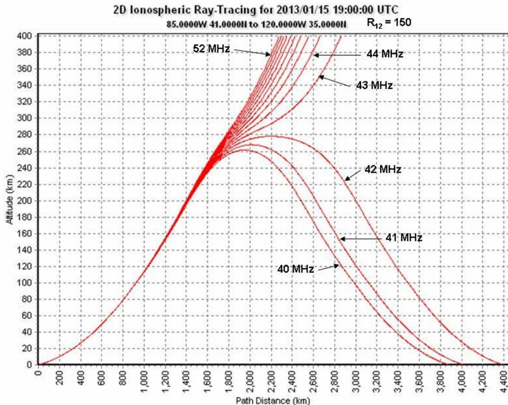
**Figure 1 – Ray traces versus frequency**
