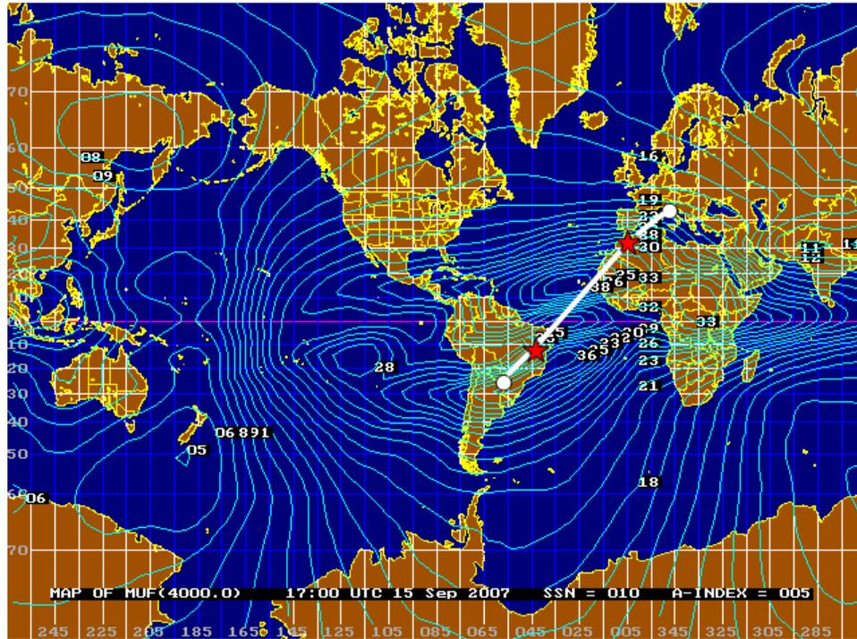
The white dot in South America is ZP6CW. The white dot in Europe is Italy. The thick white line is the short great circle path between ZP and Italy. The red 5-pointed star to the northeast of ZP6CW is an ionospheric control point 2000km out of ZP6CW. Likewise, the red 5-pointed star to the southwest of Italy is an ionospheric control point 2000km out of Italy.
