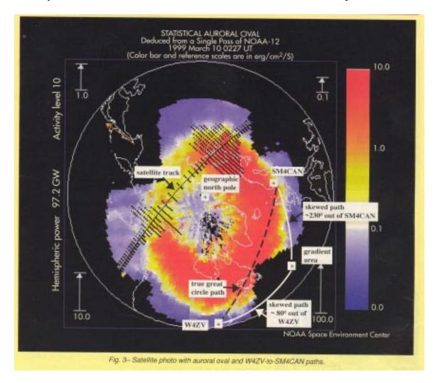
Figure 3 shows the satellite data. This is an azimuthal equidistant map with its center at the geographic north pole. The satellite track is the slightly curved line going from the southwest to the northeast just above the center of the photo. The length of the solid lines
