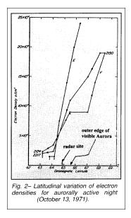
Figure 2 shows an electron density profile derived from the auroral-zone incoherentscatter radar near Chatanika, Alaska (Bates, Belon, and Hunsucker, 1973). The y-axis is electron density in electrons per cubic centimeter. The x-axis is geomagnetic latitude. The scans were along a constant magnetic longitude. The profile is for a night when the authors reported that the geomagnetic field was moderately active as evidenced by observations of the visible aurora.
